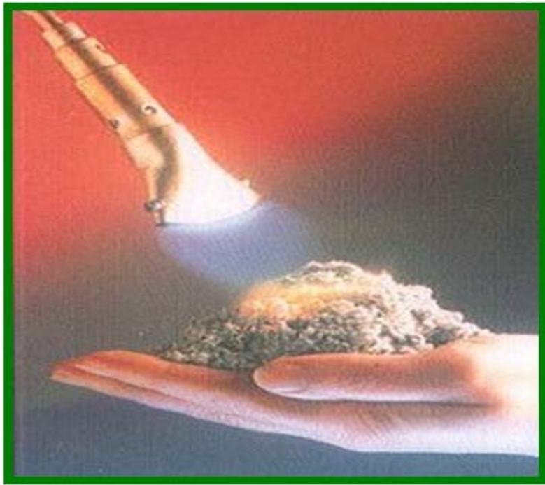
Fire retardancy and insulating ability of cellulose insulation
